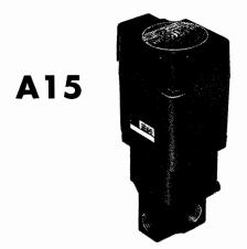
The special version of the 200 Series designed for hazardous locations has been approved by CSA for Class I, Groups B, C & D; Class II, Groups E, F & G. Maximum rated fluid and ambient temperature is 40°C; maximum pressure is 150 p.s.i. Approval is limited to certain common AC & DC voltages which are those designated in the table on the opposite page by the suffixes -11, -12, -22, -50, -55, -60, -61.
