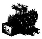
The 35 series is the most versatile solenoid valve in this group. It has an all molded encapsulated coil and can be supplied as an individual inline, stacking or manifold base mounted valve. It is also available mounted on an extruded circuit bar® which can be machined to customers' specifications. Other options include integral pressure regulators and exhaust flow controls. This valve is also used as the pilot valve for the 4 way 82 Series.
